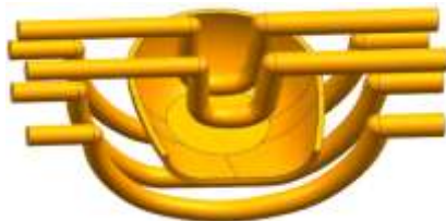
Figure 3. When D/d=1.2, the structure of the variable cross-section.
